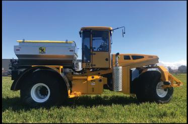
GK 3W6 self-propelled spray buggy has been designed for light-weight, high-flotation applications for both spreading and spraying. The three-wheel stance provides staggered tire spacing to limit ground pressure and compaction.
