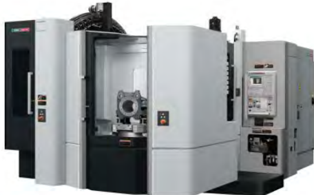
DMG MORI NHX6300 PRODUCTION MILLING MACHINE 4 axis horizontal machining center X: 41.3"/1,050mm Y: 35.4"/900 mm Z: 40.6"/1,030mm
