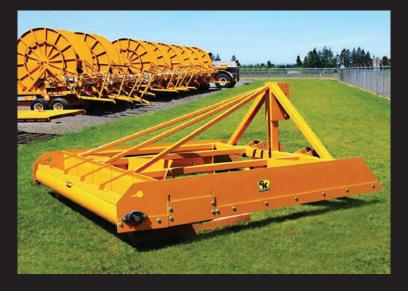
GK Orchard Levelers slice and crowd the dirt to the center then the levelers push dirt back towards the outside continuously cutting and filling. Then an adjustable V float spreads the dirt back out evenly filling in any low spots. The rear smoothing plate stabilizes dirt to firm and flatten the soil. Each unit has multiple 3-point hookups with standard and quick attachment.
