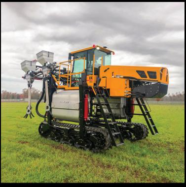
The over-the-row spray delivery system with stainless steel saddle tanks, mechanical agitation, centrifugal or diaphragm pumps, product controllers, and a variety of boom configurations and sizes will meet all of your spraying needs. From wet drops and broadcast booms, to an air blast system and granular fertilizer spreaders – the TR6 is customizable to meet your specific crop needs.
